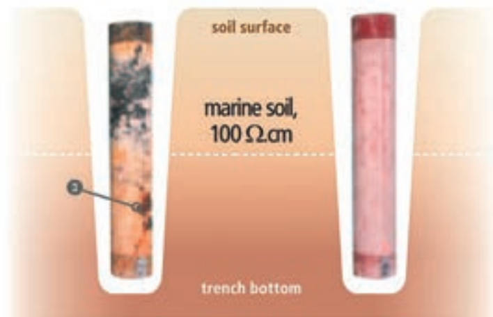
200 g/m 2 zinc + 80 µm bituminous paint coating
